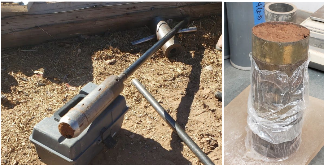
Figure 3-3: Collected sample in hand operated device (right) and sample in rings at lab (left).
