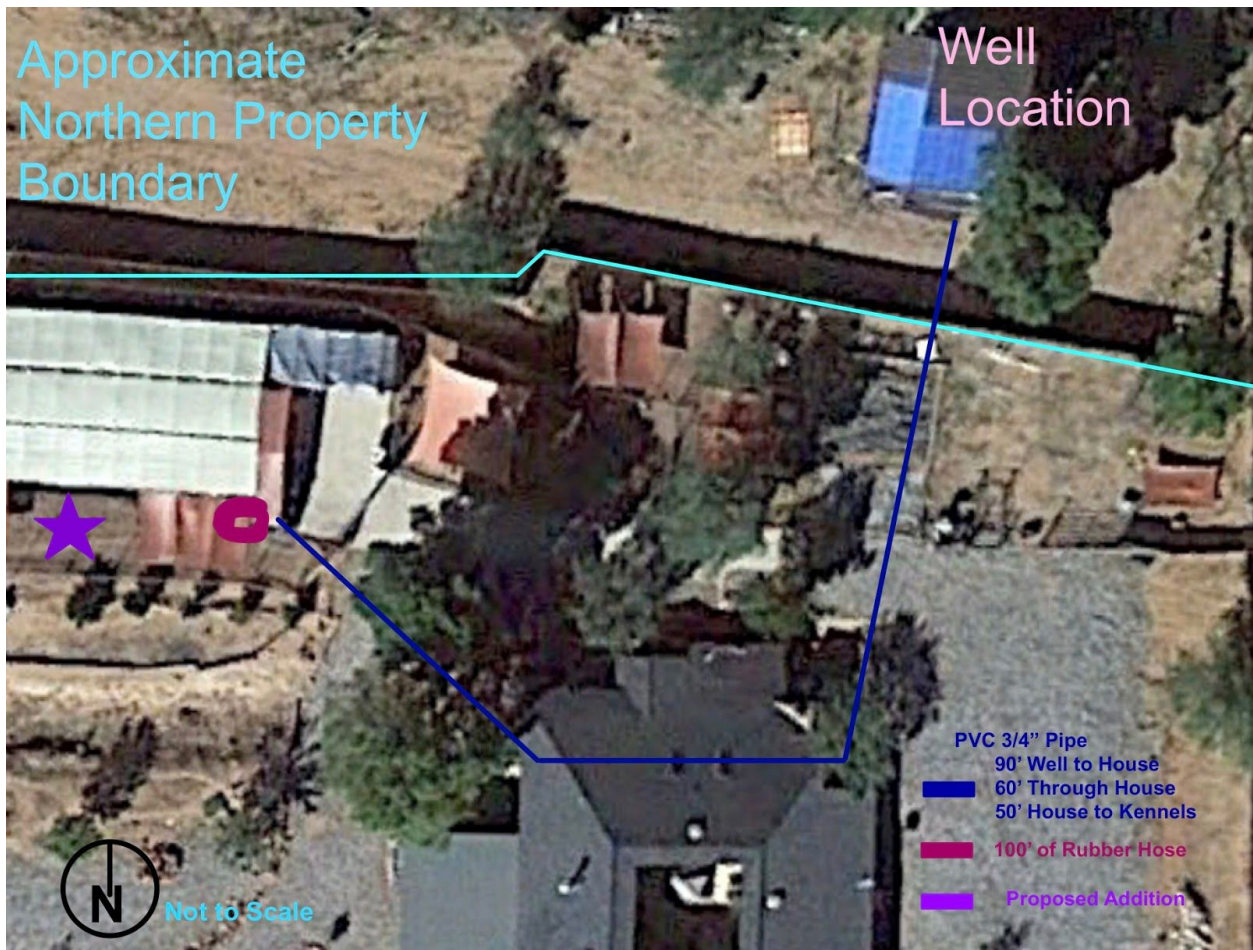
Figure 6-1: Existing well location in respect to the site location and pipe system. Star represents the general location of the project location. Figure is not to scale.
